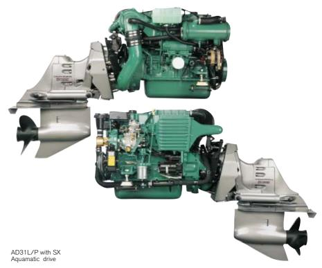
Hydrodynamic design of the lower drive housing ensures excellent course stability both at high speed and when maneuvering at low speeds and reverse.
