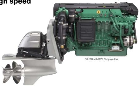
EVC works closely together with the engine management system offering you constant power output regardless of temperature (5–55°C / 41–131°F) and quality of the fuel. The system is built on the latest automotive technology with waterproof connectors, so it's just plug and go.
