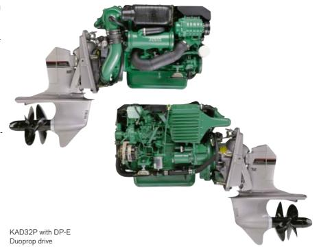
All the important service points on the engine are conveniently located at the top and the port side.
