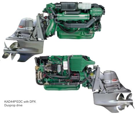
ing. Pattern-matched spiral bevel gears for optimum strength and minimum gear whine. Break-away shaft coupling to prevent costly drivetrain repairs. Engine coolant water intake on the drive. Exhaust through propeller hub, cavitation plate and transom shield for maximum quietness and low power losses.
