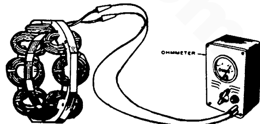
OHMMETER RESISTANCE BETWEEN F1 AND F2 SHOULD BE 12.2 OHMS (± 10%)
