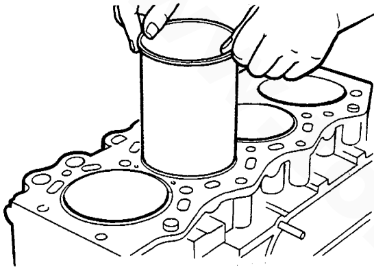
INSTALLING CYLINDER LINERS
