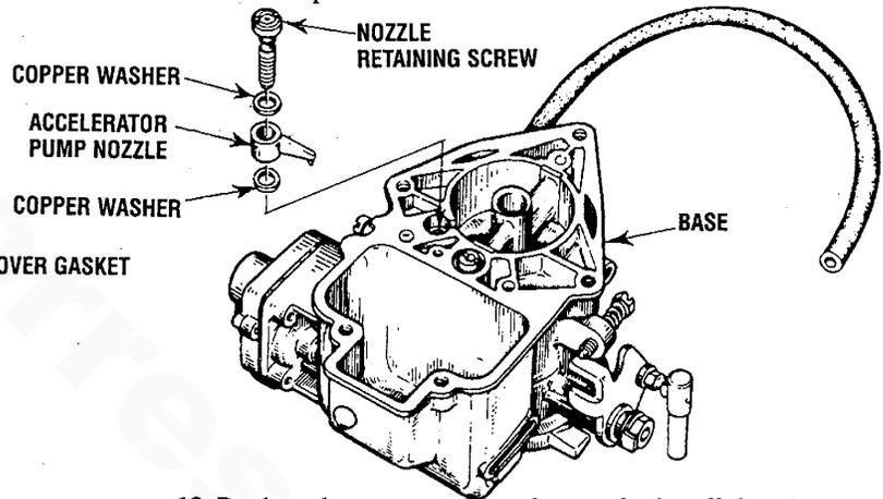
13. Replace the two copper washers and reinstall the accelerator pump nozzle. Snug down the nozzle's retaining screw. **Do not** overtighten the screw, Reinstall the accelerator pump diaphragm, spring and housing. Snug down the four retaining screws.
