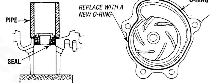
1. Install the water seal by tapping as shown above.
