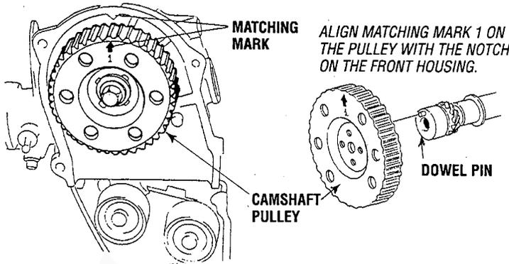
1. Install the camshaft pulley washer and lock bolt. Prevent the pulley from turning and tighten the lockbolt to the specified torque.
