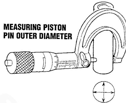
**MEASURING PISTON PIN OUTER DIAMETER**
