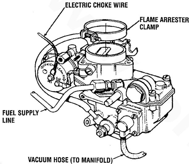
4. Remove the two choke assembly retaining screws and their washers. Disconnect the electric choke assembly from the carburetor.
