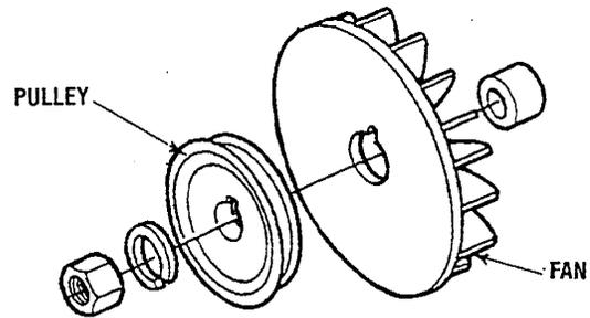
**PULLEY AND FAN COMPONENTS**
