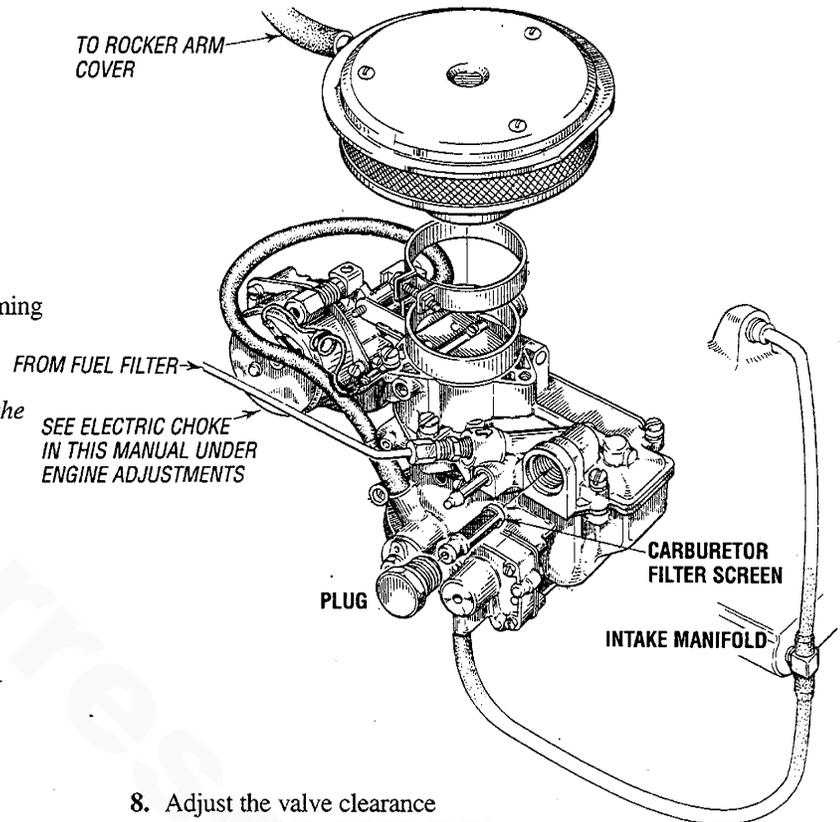
8. Adjust the valve clearance (See *ENGINE ADJUSTMENTS*)
