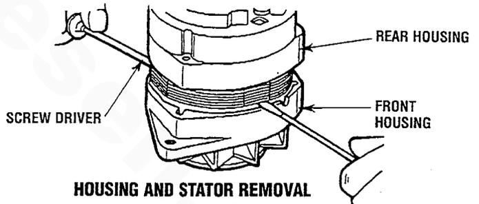
**HOUSING AND STATOR REMOVAL**
