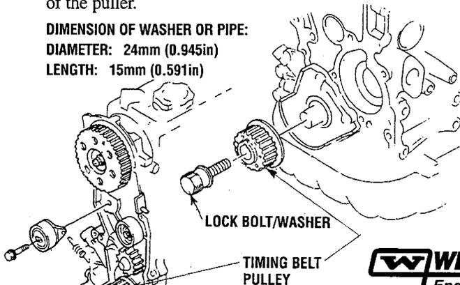
4. Screw in the pulley puller, and remove the spacer and taper ring together.
