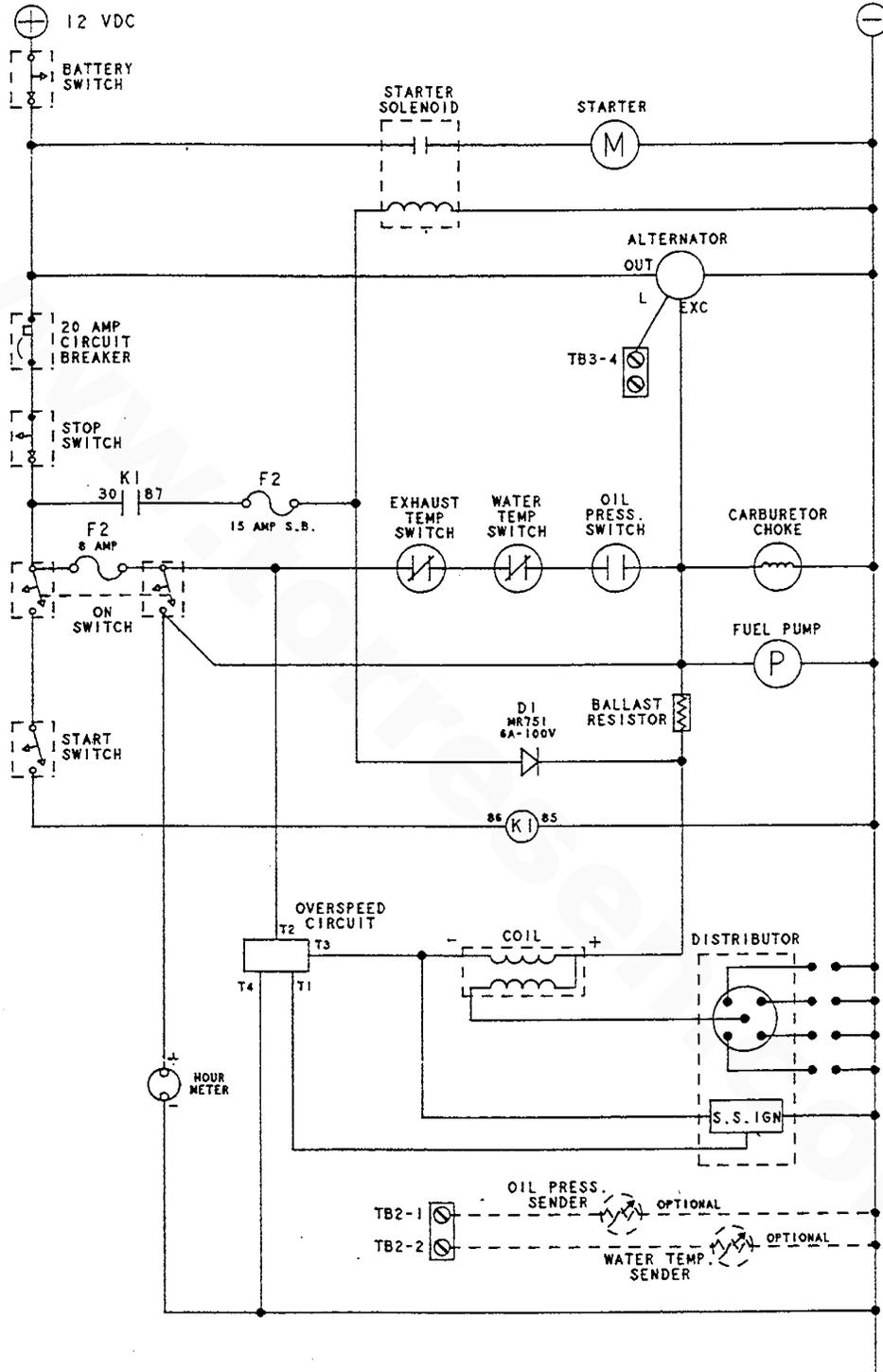
**NOTE:** The only difference between the diagrams on the two previous pages [New Generators] and these diagrams occurs at the overspeed switch [T5 to ignition].
