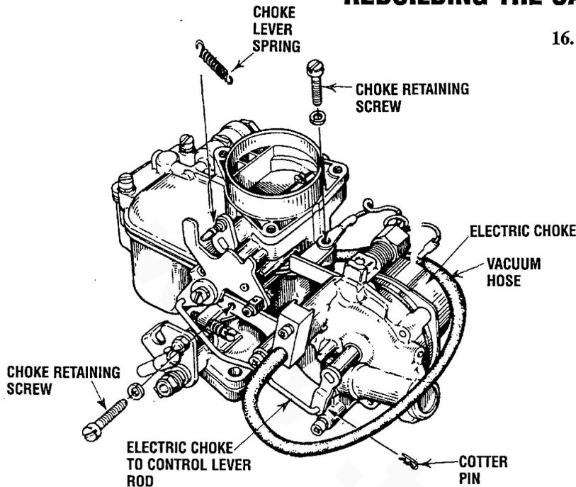
15. Reconnect the electric choke assembly to the carburetor and replace the two choke assembly retaining screws and their washers. Re-attach the electric choke to control lever rod to the electric choke assembly and insert the cotter pin. Re-attach the vacuum hose.
