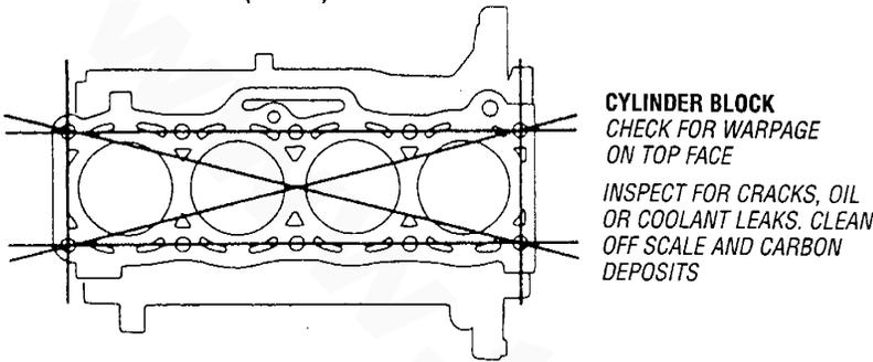
3. If the distortion exceed specification, repair by grinding, or replacing the cylinder block.
