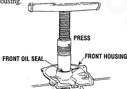
2. Set the front housing gasket in place on the engine. Coat the oil seal with fresh engine oil and install the front housing using a new gasket.
