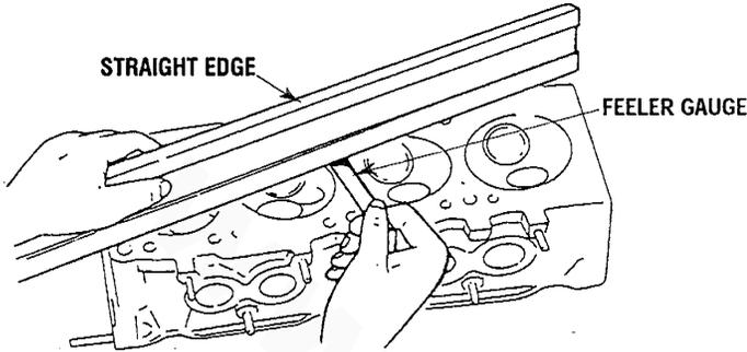
Measure the cylinder head distortion in the six directions shown below using a gauge and straight edge.
