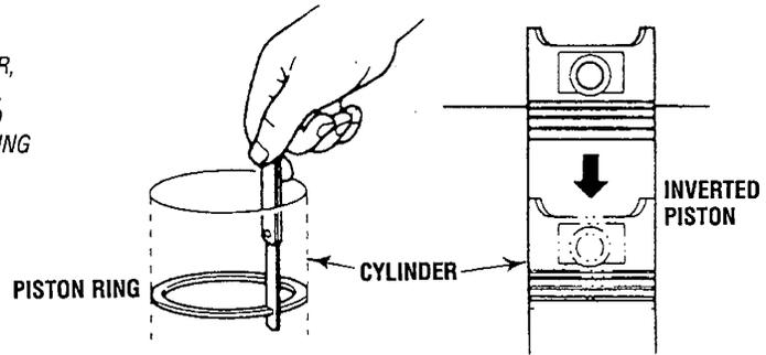
8. Measure the piston ring to ring clearance around the entire circumference using a new piston ring.
