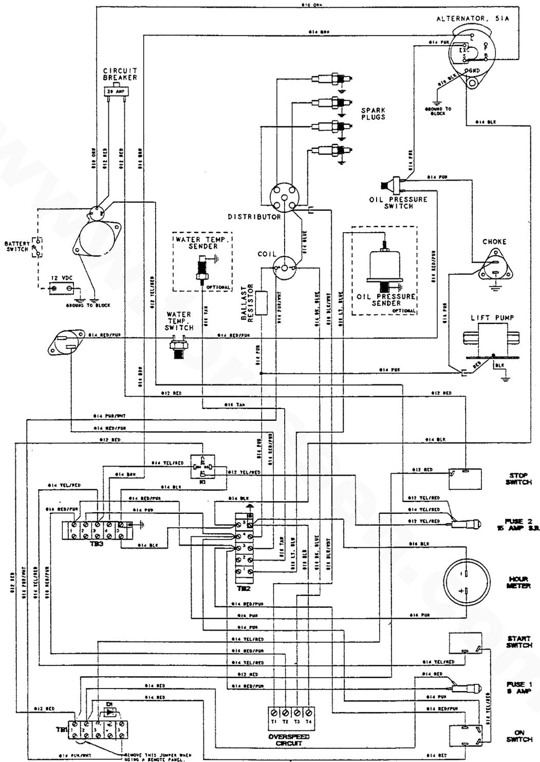
**NOTE:** The only difference between the diagrams on the two previous pages [new generators] and these diagrams occurs at the overspeed switch [T5 to ignition].
