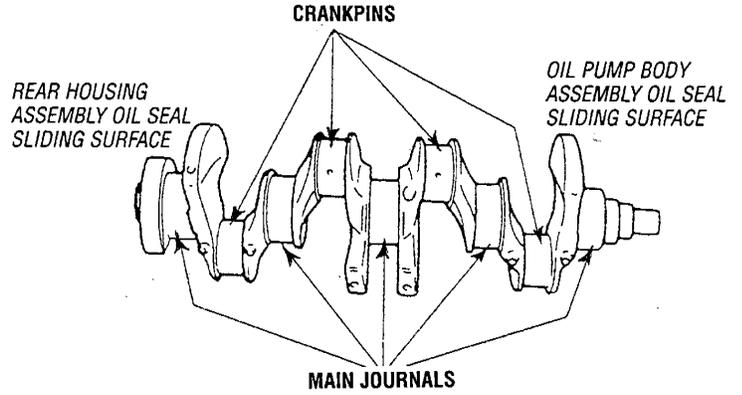
5. If the diameter is less than the minimum, grind the journals to match undersize bearings.
