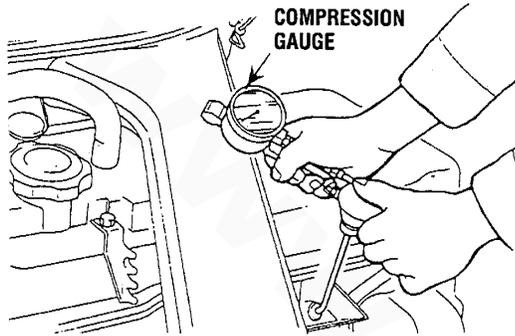
6. Connect a compression gauge to the No.1 spark plug hole.
