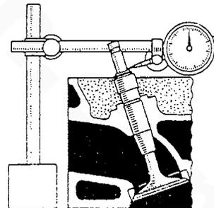
8. If the cylinder exceeds specification, replace the valve and/or valve guide.
