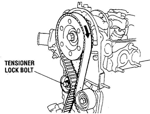
1. Loosen the timing belt tensioner lock bolt and apply spring tension to the belt.
