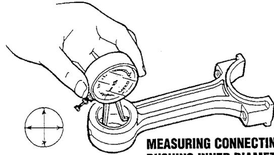
**MEASURING CONNECTING ROD BUSHING INNER DIAMETER**
