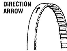
IF RE-USING THE TIMING BELT, INSTALL IT IN THE DIRECTION OF THE APPLIED ARROW - FORWARD ROTATION.
