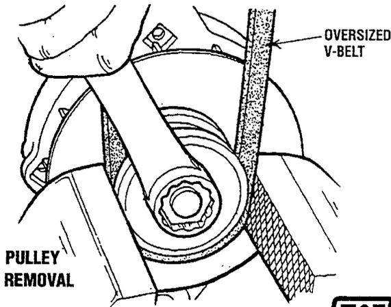
10. Place an oversized V-belt around the pulley and fasten the pulley in a vise.
