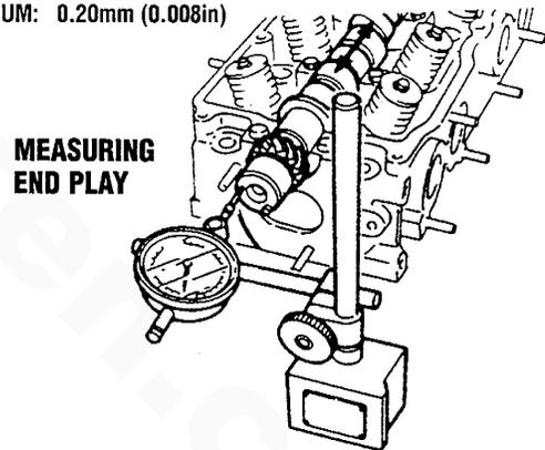
**NOTE:** If the end play exceeds specifications, replace the camshaft and/or cylinder head.
