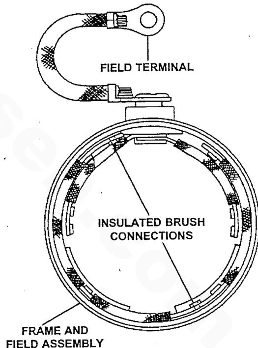
FIGURE 10. FRAME AND FIELD ASSEMBLY
