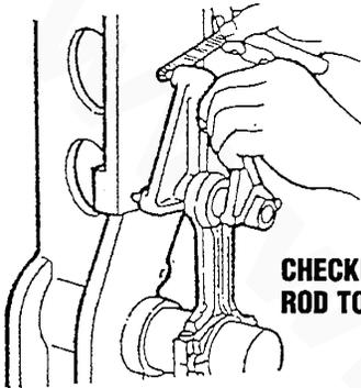
**CHECKING CONNECTING ROD TORSION LIMIT**
