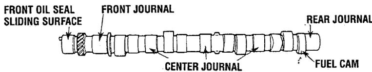
5. Check the camshaft runout. Replace if necessary. Set the front and rear journals on V-blocks and rotate the camshaft one full turn to measure deflection (runout).
