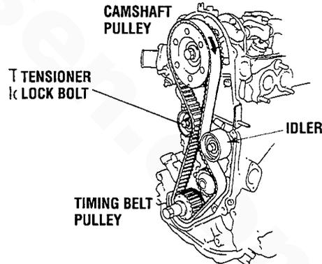
14. Remove the camshaft pulley. Remove the pulley by inserting a T-wrench or similar tool to prevent it from turning.
