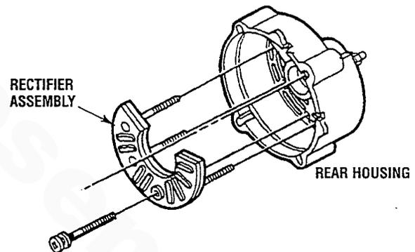
6. Assemble the front and rear housings as follows:
