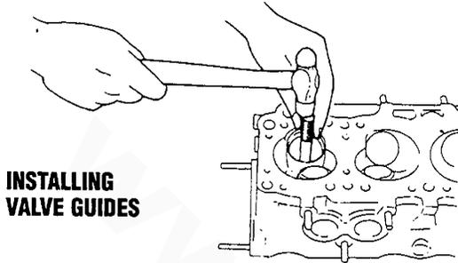
**INSTALLING VALVE GUIDES**
