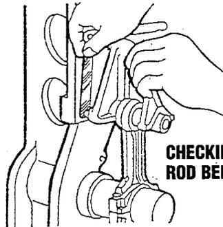
**CHECKING CONNECTING ROD BENDING LIMIT**
