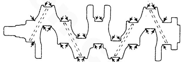
**ALWAYS CHAMFER THE POINTS MARKED WHEN GRINDING THE JOURNALS AND PINS**
