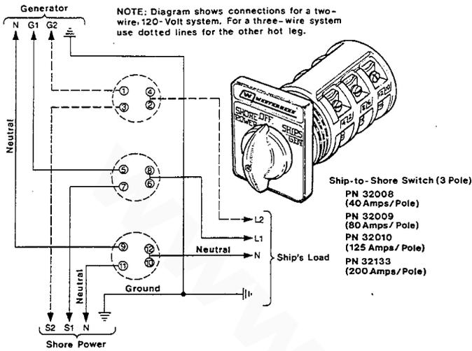
If the installer connects shore power to the vessel's AC circuit, this must be done by means of the Shore Power Transfer Switch. Set the transfer switch shown in the diagrams to the OFF position. This switch prevents simultaneous connection of shore power to generator output.
