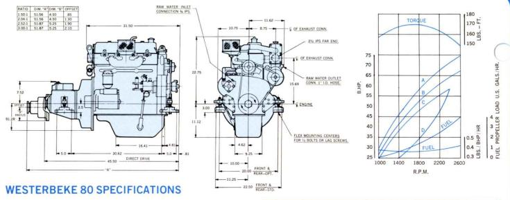
**Type:** Direct injection, naturally aspirated, four cycle, four cylinder in line, fresh water cooled marine diesel engine.
